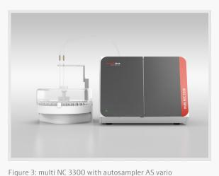
automated measurement process for large sample sequences is supported by a wide range of available autosamplers with integrated sample homogenization, ranging from 21 sample positions (AS 21hp) to 147 sample positions with the AS vario and AS vario ER for the multi N/C 3300. The AS 60 autosampler for the multi N/C 2300 also offers a very good level of automation for sewage plant testing laboratories.
