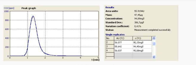
Figure 2: Typical measurement curve and replicate results for the investigated cellulose suspension
