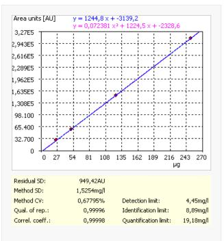
Figure 1: Calibration curve and method characteristics
